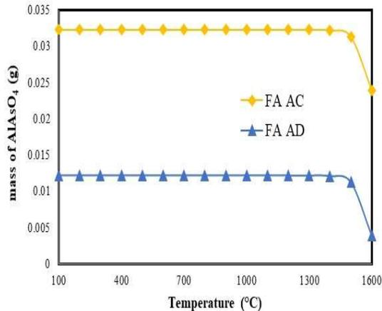
Figure 1: Prediction of As-bearing compound during combustion of Fly ash AC and AD
