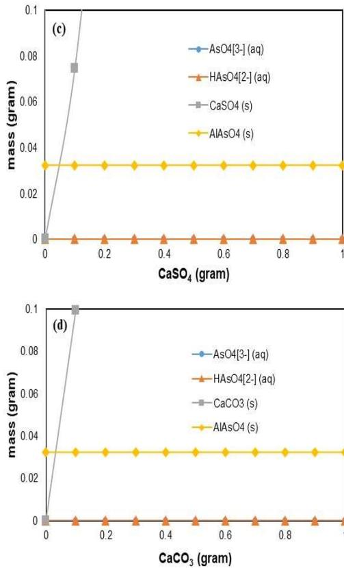
Figure 2: Effect of calcium compounds into arsenic leaching process on FA AC at 25 °C atmospheric condition (a) CaO, (b) Ca(OH)<sub>2</sub> (c) CaSO<sub>4</sub> and (d) CaCO<sub>3</sub>
