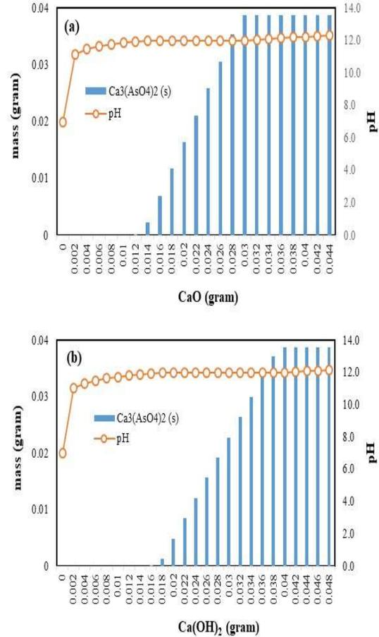
Figure 3: Effect of inhibitors into leachate pH on arsenic leaching process on FA AC at 25 °C atmospheric condition (a) CaO and (b) Ca(OH)<sub>2</sub>
