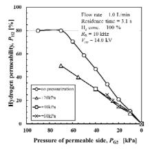
Fig. 2 Hydrogen separation characteristics of PMR at various differential pressure.
