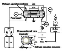
Fig. 1 Configurations of plasma membrane reactor and the experimental setup.
