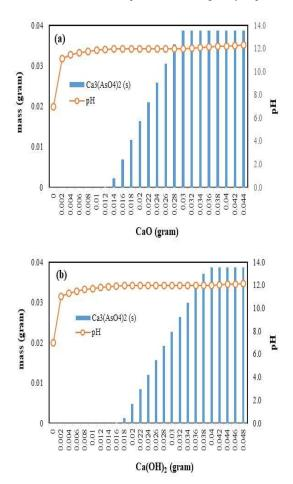
Figure 3: Effect of inhibitors into leachate pH on arsenic leaching process on FA AC at 25 °C atmospheric condition (a) CaO and (b)  $Ca(OH)_2$
