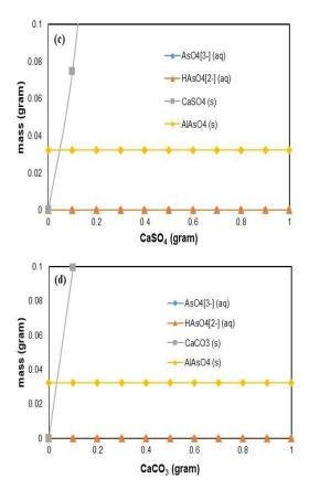
Figure 2: Effect of calcium compounds into arsenic leaching process on FA AC at 25 °C atmospheric condition (a) CaO, (b)  $Ca(OH)_2$  (c) CaSO<sub>4</sub> and (d) CaCO<sub>3</sub>
