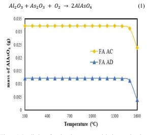
Figure 1: Prediction of As-bearing compound during combustion of Fly ash AC and AD
